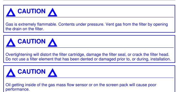
Fuel filters are required equipment on all Cummins® natural gas engines. They are designed to remove oil and harmful particles from the fuel before they damage the fuel system or other engine components. These filters are a coalescent type filter that will capture the oil contaminants and moisture typically found in natural gas.
