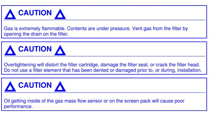
Fuel filters are required equipment on all Cummins® natural gas engines. They are designed to remove oil and harmful particles from the fuel before they damage the fuel system or other engine components.
