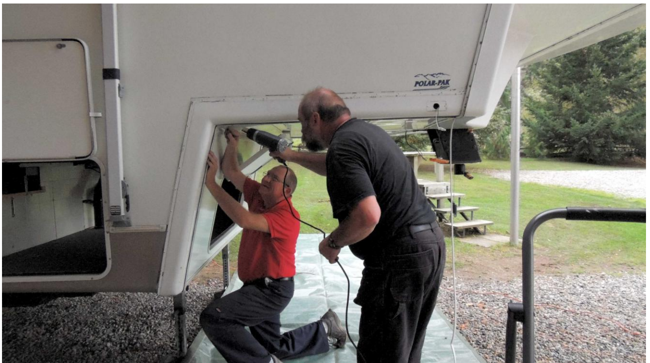
With the help of friend, a heat gun and a putty knife we take off the corner elements.
